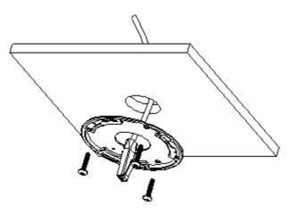
Fasten the camera to ceiling by turning clockwise direction
