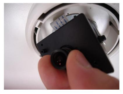
Attach the dome cover to the camera and push it into the groove until it clicks.
