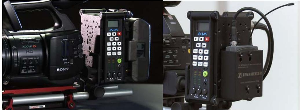
**Camera Mounting Examples Using Optional Mounting Plate**
