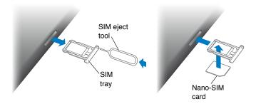
Open the SIM tray. Insert a SIM eject tool (sold separately) into the hole on the SIM tray, then press firmly and push the tool straight in until the tray pops out. Pull out the SIM tray to install or replace the SIM card. If you don't have a SIM eject tool, try the end of a small paper clip.
