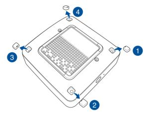
4. Remove the four screws securing the cover.
