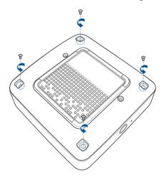
5. Get one screw from the ones you previously removed then place it into the hole. Leave a portion of the screw head that would be enough for you to hold.
