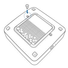
6. Hold the screw then gently pull out the cover from the bottom side of the VivoMini. Use your other free hand to hold the VivoMini in place.
