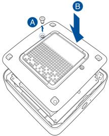
9. Reattach the screws to secure the cover back on the bottom side of the main box.
