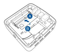
8. Remove the screw you previously attached on the bottom cover (A), then align and insert the bottom cover back on your VivoMini (B)
