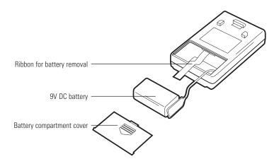
**Note:** To avoid possible damage due to leakage, the batteries should be removed if the PRO 88W will not be used for a long time.
