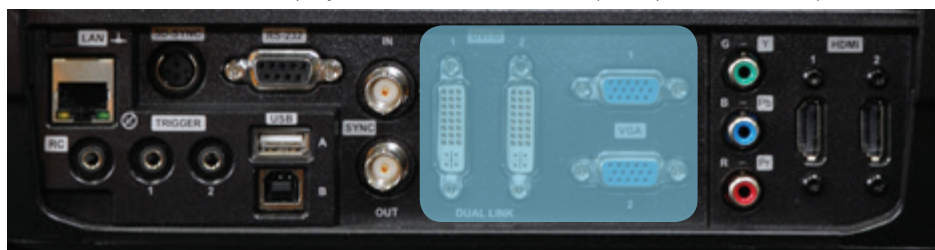
Figure 5-5. Connecting a computer source
