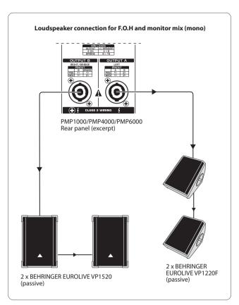
Fig. 5.3: Dual mono operation
