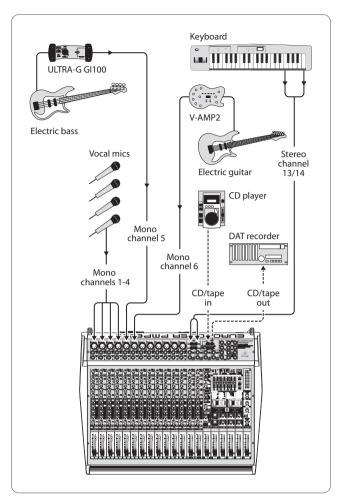
Fig. 5.4: Standard set-up (example)
