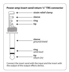
Fig. 4.5: Stereo ¼" TRS connector for power amp ISR connection
