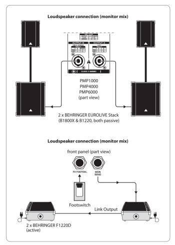
Fig. 5.1: Stereo operation
