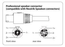
Fig. 4.6: Professional speaker connector with polarity allocation
