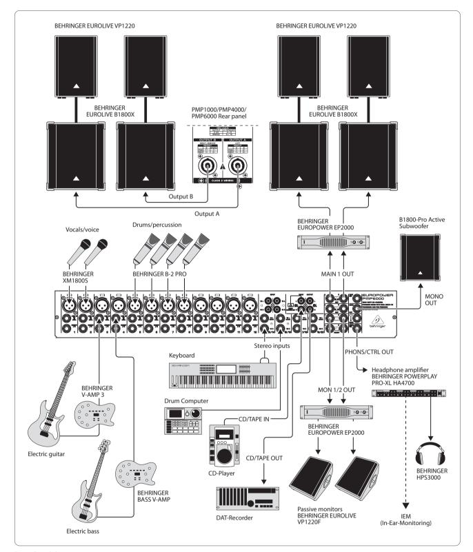
Fig. 5.5: Expanded set-up
