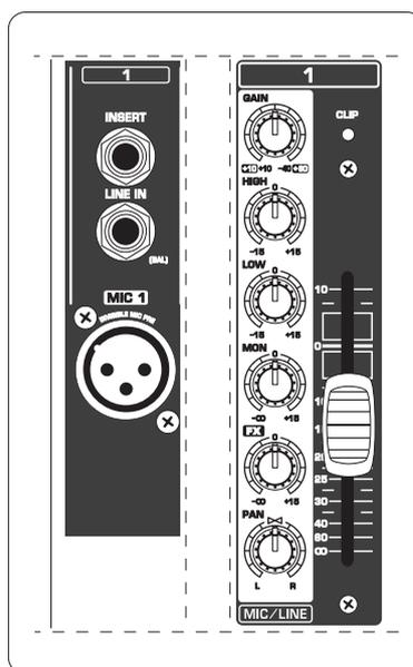
Fig. 2.1: Connectors and controls on the mono channels
