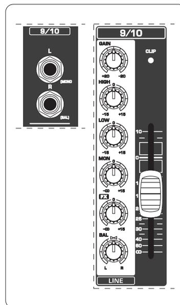
Fig. 2.2: Connectors and controls on the stereo channels
