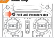
**NOTICE:** Do not press the Motor Stop button while the aircraft is airborne. The motors could stop, causing the aircraft to crash
