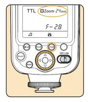
**Using the flash with wide-angle lenses:** When you have a lens wider than 24mm mounted on your camera, you can use the built-in diffuser panel to give the flash an angle of coverage equivalent to that of an 18mm lens.
