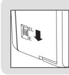
Move the mode selector switch on the back of the P-touch labeler to the "E" position before connecting the USB cable.
