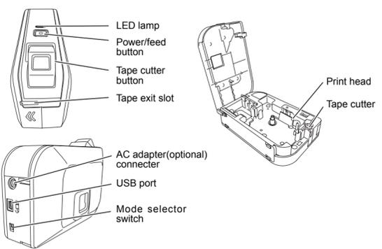
The PT-1230PC has 2 mode selector settings - "EL" and "E". The mode selector switch is pre-set at the factory to the EL mode, for use with P-touch Editor Lite. For E mode, you need to download P-touch Editor 5.0 and the required drivers. For details on how to download the P-touch Editor 5.0, see "Starting P-touch Editor 5.0" below.
