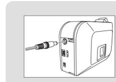
When using the optional AC adapter (AD-24ES), insert the plug on the adapter cord into the adapter jack on the bottom end of the P-touch labeler. Insert the plug into the nearest standard electrical outlet.
