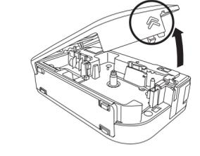
Verify that the P-touch labeler is turned off. Open the cassette cover as shown by the arrow in the above illustration while pressing the part marked "<<".
