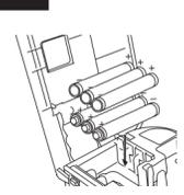
Insert six new AAA alkaline batteries (LR03), making sure that their poles point in the correct directions. Always replace all six batteries at the same time using brand new ones.
