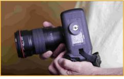
2. Attach the Camera Hub by FIRMLY THREADING it into the 1/4" tripod mount of your camera. You must ensure this is REALLY TIGHT! Recheck frequently!
