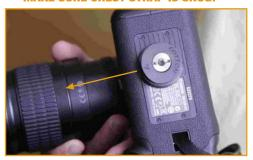
3. Ensure you align the arrow on the Camera Hub in the direction of the lens.
