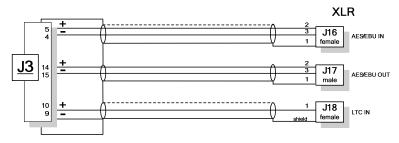
**Note:** digital cable for VX222HR with additional AES/EBU Sync input on special request.
