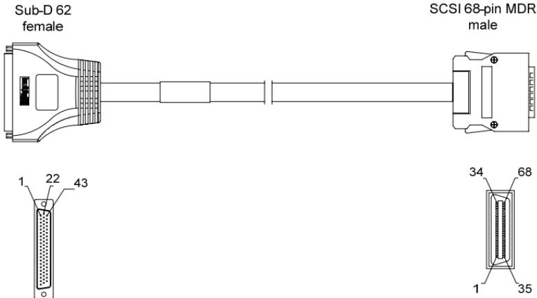
If your card is a VX442e, i.e. has a PCI EXPRESS™ (PCIe®) bus, use this adapter cable to connect the audio I/O cable with the card.
