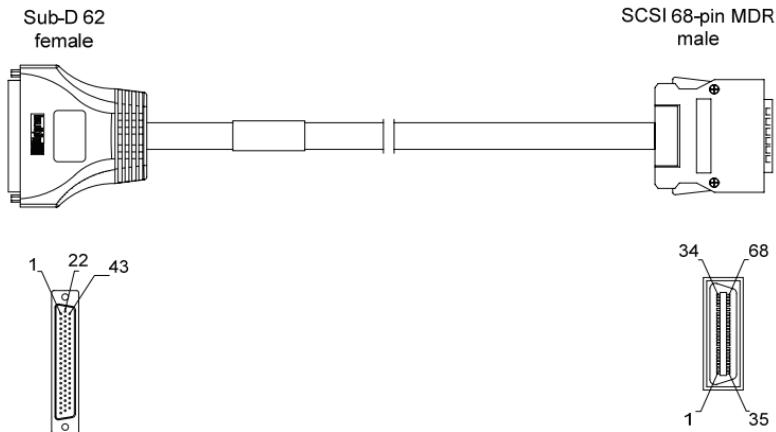
Use this adapter cable to connect the VX881e cable with the card.
