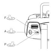
P mode (Positioning) : P mode works best when GPS signal is strong. There are three different states of P mode, which will be automatically selected by the Inspire 1 depending on GPS signal strength and Vision Positioning sensors:
