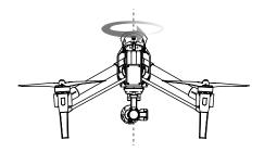
Hold the aircraft vertically with nose pointing downward, and rotate it 360 degrees around the center axis. Recalibrate the compass if the Aircraft Status Indicator show solid red.
