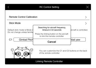
Locate the Linking button on the front of the aircraft, as shown in the figure shown below. Press the Linking button to start linking. The Remote Controller Status Indicator will display solid green if Link is succeed.
