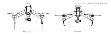
The Front and Rear LED show the orientation of the aircraft. The Front LED displays solid red and the Rear LED displays solid green.
