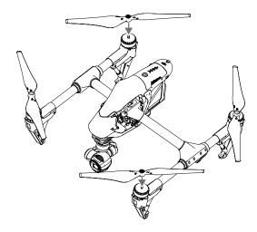
A Place all propellers onto the correct motor and tighten by hand to ensure security before flight.
