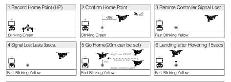
▲ Aircraft cannot avoid obstruction during the Failsafe RTH, therefore it is important to set an reasonable Failsafe altitude before each flight. Launch the DJI Pilot app and enter "Camera" view and select "MODE" to set the Failsafe altitude.
