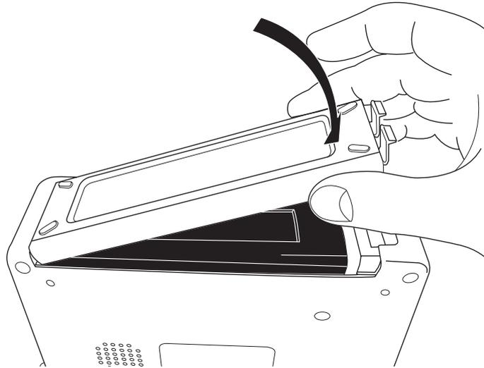
**<Note>**: Wipe terminals of the battery case and batteries with a dry cloth on occasion. If terminals are dirty, the voltage supplied to the unit may drop down.
