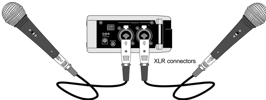
The FR-2LE provides the HPF (high-pass filter) and limiter functions which are useful for recording using external microphones. It also provides +48V phantom power capability for condenser microphones. See pages 55 and 92 for details about HPF and limiter on/off settings. See page 95 for details about phantom power on/off setting.
