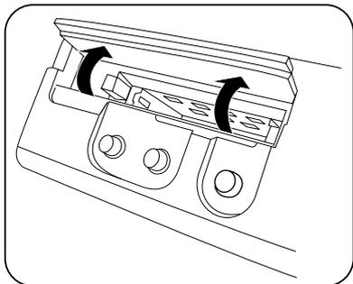
When opening the slot protection cover on the front panel, you can see the slot and eject button inside.
