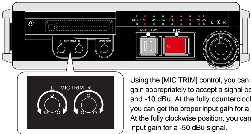
Using the [MIC TRIM] control, you can adjust the input gain appropriately to accept a signal between -50 dBu and -10 dBu. At the fully counterclockwise position, you can get the proper input gain for a -10 dBu signal. At the fully clockwise position, you can get the proper input gain for a -50 dBu signal.
