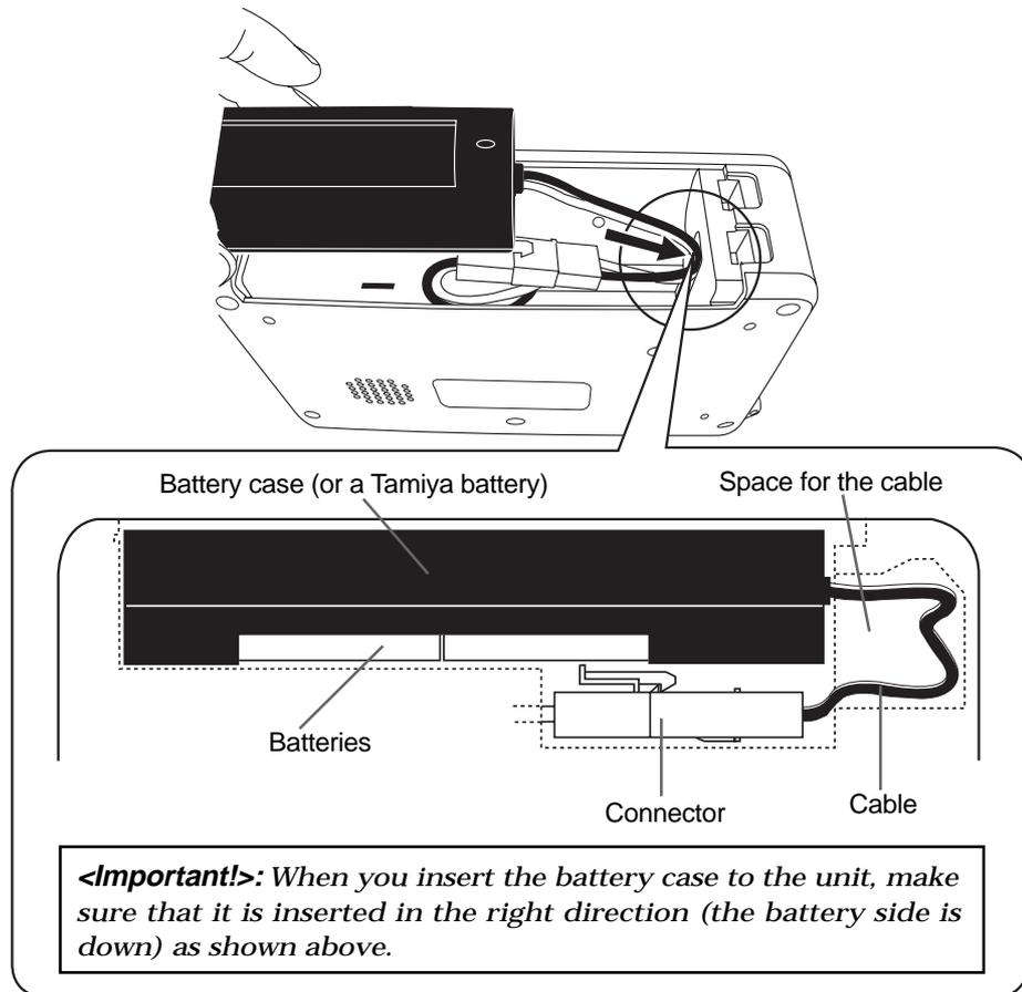
**<Important!>** When you insert the battery case to the unit, make sure that it is inserted in the right direction (the battery side is down) as shown above.
