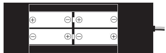
**Setting the battery case (or a Tamiya battery) to the unit**
