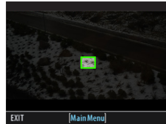
White Balance Shot screen appears after test capture to illustrate the area chosen for white balance calculation.
