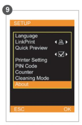
About: It displays information about the current printer firmware, color table version, and controller firmware version.
