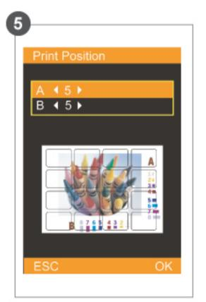
Based on the printout of 4x4 or 4/2/4 sticker, adjust the parameters in the A and B column if needed, then press [OK] to save values.
