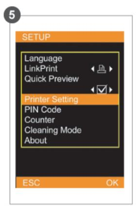
Printer Setting: Allows users to enable or disable Auto-Color and Matte effect, adjust LCD screen, color setting, and print position.
