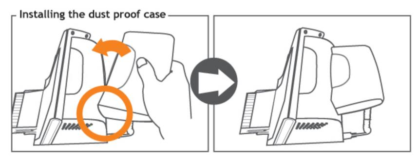
Gently insert the latch into the corresponding latch receiver opening on one sid first, then gently push the latch on the opposite end of the dust proof case into the corresponding latch receiver opening to finish the installation.
