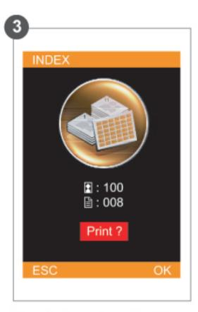
The printer automatically counts the copy of prints based on the index format. Please press [OK] or [PRINT] to start printing or press [ESC] to go back.
