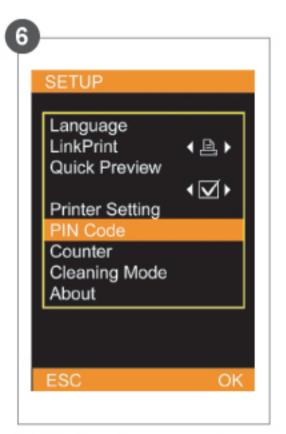
PIN Code: To assure printer security, a PIN code can be set. Once set, the PIN code would have to be entered when the printer reboots or the printing list is being cleared.
