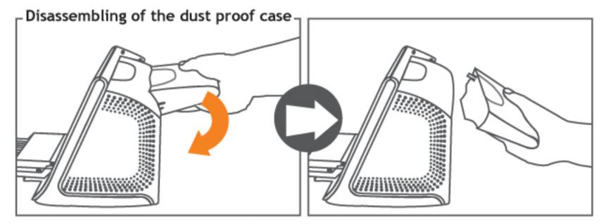
Hold the end of dust proof case firmly and gently push the dust proof case downward to uninstall the dust proof case.
