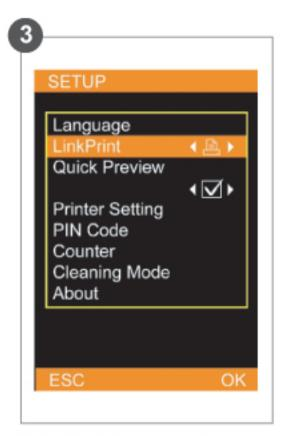
LinkPrint: Users are allowed to control the S420 by using the LCD controller or by using a digital camera.
