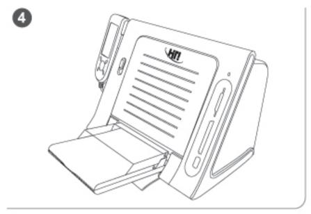
Close the ribbon door to complete the ribbon installation.
