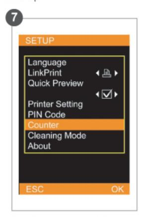
Counter: The user is allowed to reset the counter if the PIN code is correctly entered.
