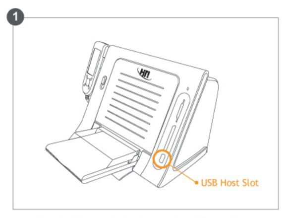
Plug the Bluetooth dongle into the USB Host Slot.
