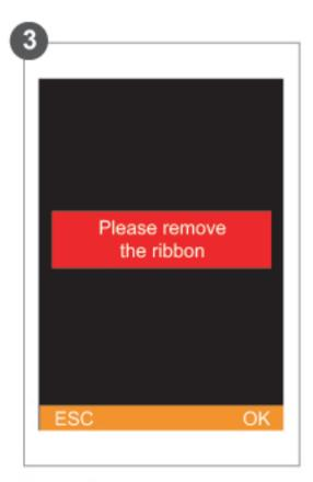
Before the cleaning process begins, please remove the ribbon cartridge from the printer and press [OK] to start the cleaning job.
