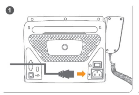
Plug the power cord into the power cord socket at the back of the printer.
