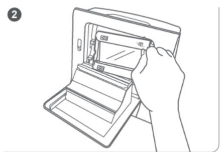
Install the ribbon cartridge inserting the left (indicated by the arrow) side of the ribbon first followed by the right side.
