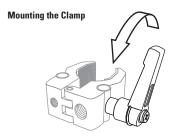
With the handle of the Atom Clamp facing you, loosen the clamp by turning the handle counterclockwise.
