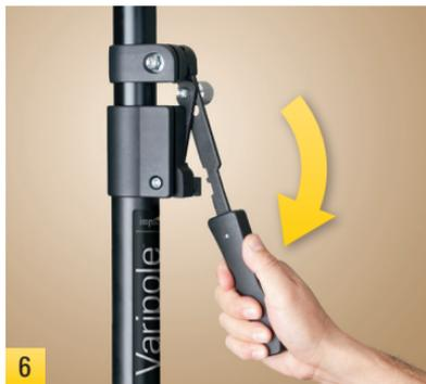
Making certain that the Varipole is vertically level, bring the handle back down until it clicks into its locking latch.
