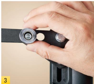
Slide the tension knob to the lower (more tension) or upper (less tension) position on the handle bracket. Retighten the tension knob and return the handle to its locked position.
