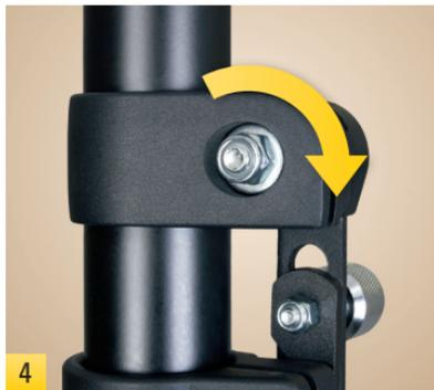
If the upper tube slips under the stress of your installation, use a socket wrench to tighten the nut at the top of the handle bracket.
