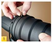
The snoot slides over the slave flash's accessory flange. Tighten the mount screw.
