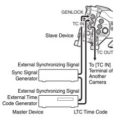
Input the external synchronizing signal to the external time code generator and the [GENLOCK] terminal of this camera recorder.
