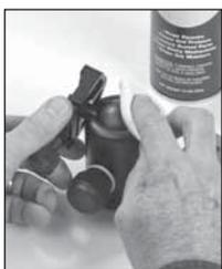
We recommend cleaning your head every 4-6 weeks. To do this, loosen the main control knob and the tension knob. Move the ball into the 90 degree position. Now with a cloth lightly moistened with WD40 slowly turn the ball in the socket. When you're done with this process please wipe off any excess WD40 with a clean cloth. Also please avoid using any cleaner
