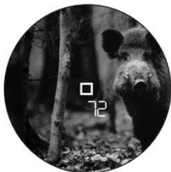
The Leica Geovid HD-R can also be used for measurements in continuous mode (Scan mode): Press the main/trigger button once, then press again and hold depressed. After approx. 2.5 seconds, the device switches to Scan mode and then performs measurements permanently. This is indicated by alternating displays:
