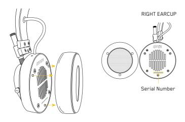
Ear pads are magnetized for easy removal/replacement. Simply grab the outside ring of the ear pad and remove. Reattach ear pads by aligning the three guide posts on the earcup with the three guide holes on the inside of the ear pad.
