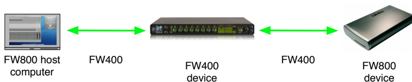
Figure D.2: Incorrectly Mixed FW800/400 Chain
