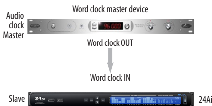
Figure 4-9: Slaving your MOTU device (a 24Ai in this example) to word clock. For the 24Ai clock source, choose 'Word Clock In'.
