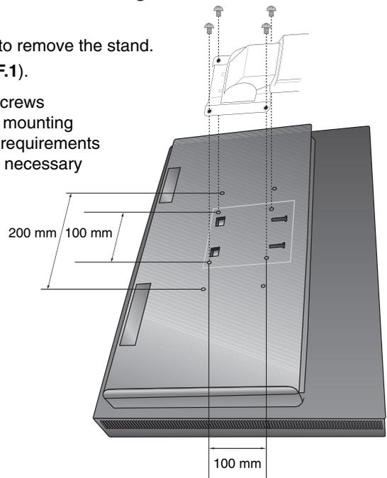
Weight of LCD assembly: 14.2 kg
