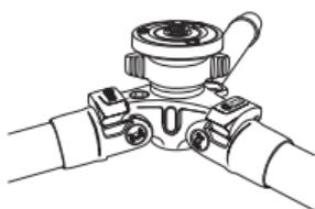
2. Turn the center column locking knob counterclockwise to unlock the center column. Remove the center column from the tripod.
