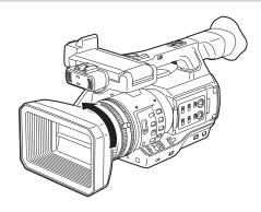
1 Rotate the lens hood counter-clockwise.
