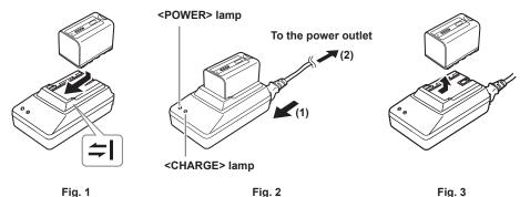
1 Place the battery horizontally along the = I mark in the battery charger and slide it in. (Fig. 1)
