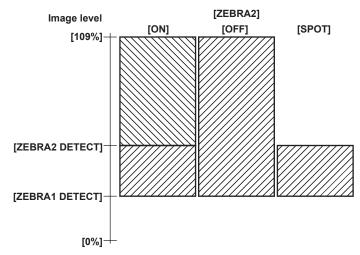
To display the zebra patterns in the video of the monitor output terminal (<SDI OUT>, <GENLOCK IN/VIDEO OUT>, <HDMI OUT>), set in the main menu  $\rightarrow$  [OUTPUT SEL]  $\rightarrow$  [VIDEO OUT ZEBRA].
