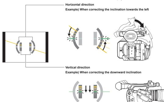
Yellow lines will be displayed when inclined. Green lines will be displayed when there is almost no inclination. Inclinations will be displayed up to approximately ±45° in the horizontal direction, and up to ±30° in the vertical direction.
