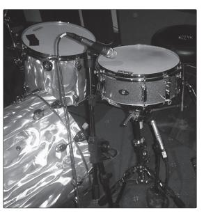
Point a dynamic microphone at the center of the snare, making sure it is placed so that the drummer will not hit it. Place a small-diaphragm condenser microphone under the drum, pointed at the snares. Experiment with the placement of both microphones. Also experiment with inverting the phase of the bottom microphone. This technique can be used in live applications.
