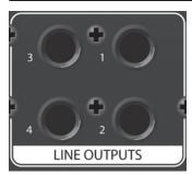
Line Outputs (AudioBox 44VSL Only). The AudioBox 44VSL has four line outputs to route to external devices, such as headphone amps and DJ mixers. Outputs 1 and 2 share their playback streams with the Main Outs and the headphone output. Outputs 3 and 4 have independent playback streams.
