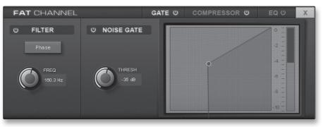
**AudioBox 44VSL Users:** You can switch between different dynamics processors by using the buttons located on the left side of this window. To close the window, click on the "X" in upper left corner.
