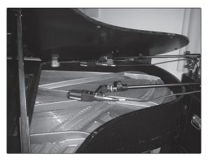
Place one microphone above the high strings and one microphone above the low strings. Experiment with distance (the farther back the more room you will capture). This technique can be used for live and studio applications.
