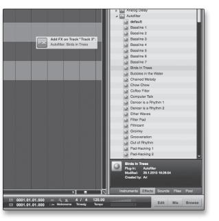
To add a plug-in effect to a track, click the Effects button and select the plug-in or one of its presets in the effects browser, then drag the selection over the track to which you would like to add the effect.
