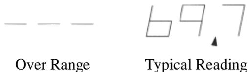
The display will stay lit for a few seconds, after releasing Measure, with the last reading frozen in the display.
