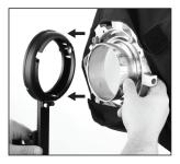
Rotate the speed ring clockwise slightly until it gently clicks into place.
