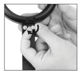
3 Slide the riser into the flash bracket's riser mount. The safety screw must be loosened enough to allow the riser to slide on the bracket. Once the riser is in place, tighten the safety screw to secure. Tighten the riser mount locking knob to fully secure it in place.
