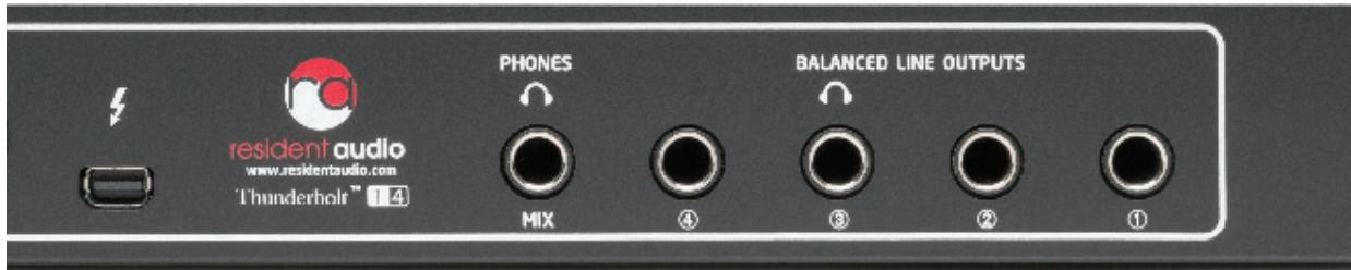
The four line-level output connectors on the rear panel of the T4 are all balanced ¼" TRS jacks. Outputs 1 & 2 are the main monitor outputs and should be connected to power amplifiers, self-powered speakers, or two channels of a mixing board. Outputs 3 & 4 can be connected to two additional input channels of a mixing board, or Output 3 can be used on its own, in which case it functions as a secondary stereo headphone jack. (For more information, see Headphones on page 9 in this manual.)
