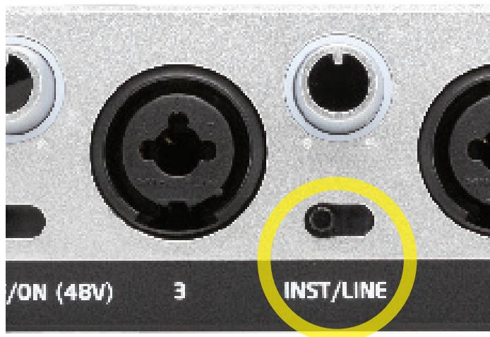
Note that the setting of the INST/LINE switch affects input monitoring even when only microphones are connected to the T4. In this case, set the INST/LINE switch for each pair to LINE if you want to monitor the incoming mic signal(s) in stereo, or to INST if you want to monitor in mono.
