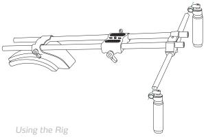
With the camera mounting plate, shoulder pad, and dual grips assembled, place the rig on your shoulder. Slide the shoulder pad until it's in a comfortable position in relationship to the dual grips. When the shoulder pad is in position, tighten the orange thumb-screw securely to lock it in place.
