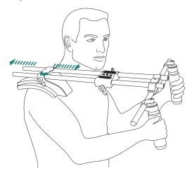
Place the camera on the camera mounting plate, using the 1/4" or 3/8" screw. Be careful to maintain balance so the rig doesn't fall over. Withdraw the other two camera mounting screws enough so the camera will sit flat on the camera mounting plate. Tighten the camera mounting screw securely. An Allen wrench is supplied for tightening the camera mounting screw.
