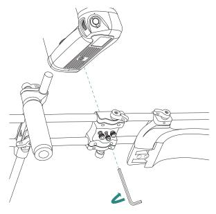
3 Slide the camera mounting plate with the camera on it on the rails until the camera is in the position you desire. Tighten the orange thumb-screw securely.
