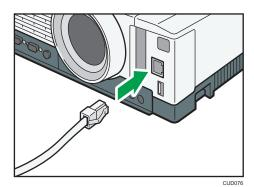
Connect the other end of the Ethernet cable to a network device such as a hub.
