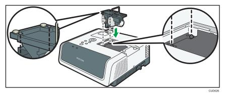
Make sure that the small projections inside the projector are inserted into the holes of the lamp unit properly.
