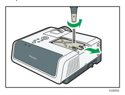
3. Loosen the two screws on the left side of the lamp unit.
