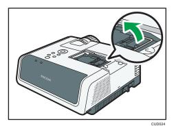
5. Hold the handle, and then pull the lamp unit out of the projector.
