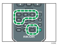
The ID number assigned to the remote control is changed to the number you pressed.
