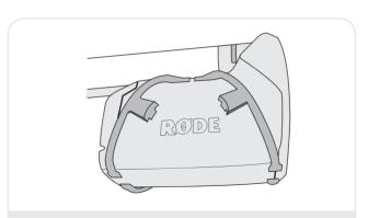
Figure 8 - Insert both ends of each band into the mic body, aligning the tapered squares in the middle of the bands to face inwards.
