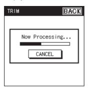
The trimmed project will be saved as a new project. In this case, the new project will have "-1" automatically appended to its name. The original project will remain unchanged. If the original project is named R26\_0001.PJT, the trimmed project will be created with the name R26\_0001-1.PJT.
