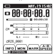
With the factory settings, the R-26's power will automatically be switched off 30 minutes after you stop playing or operating the unit. If you don't want the power to turn off automatically, change the "Auto Off" setting to "OFF" as described on p. 94.
