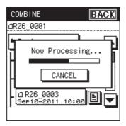
The combined project will be saved as a new project. In this case, the new project will have "-1" automatically appended to its name. The original project will remain unchanged. If the original project is named R26\_0001.PJT, the combined project will be created with the name R26\_0001-1.WAV.
