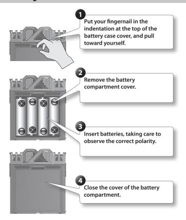
After you've installed batteries, use the "SYSTEM SETUP" menu (p. 94) to specify the type of batteries you're using.
