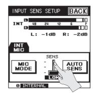
If you're adjusting multiple recording sources when using 4 channels or 6 channels, touch the tab for the recording source that you want to adjust, and then touch the <SENS> slider.
