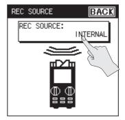
3. Touch the desired combination of recording sources.
