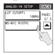
\* The <MS-MIC WIDTH> setting is shown only if the input type is set to MS mic.
