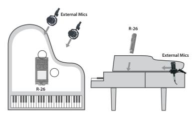
Use the internal mics to capture the sound of the strings, and use two condenser mics connected to the ANALOG IN 1/L jack and ANALOG IN 2/R jack to capture the sound from the soundboard.
