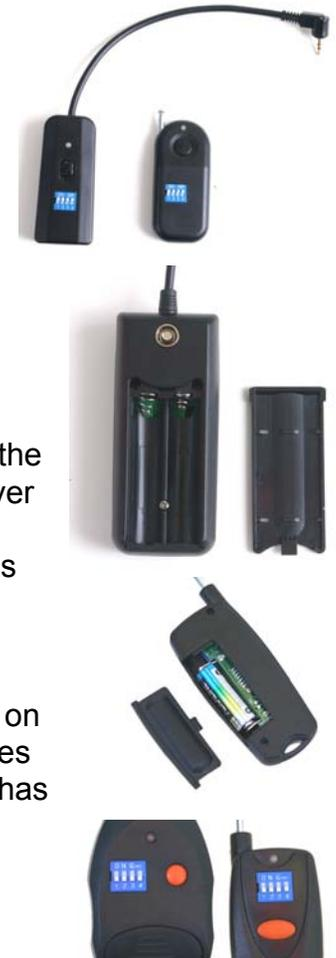
DIP Switches must be set the same on both transmitter and receiver
