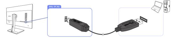
Connect the USB cable to [  $\square$  ] on the back of the product and USB [  $\square$  ] on the PC.
