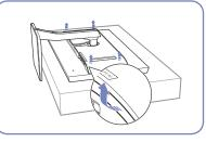
Remove the rear cover by pulling the corners in the direction of the arrows.
