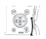
\* The shutter speed of some Samsung NX cameras changes automatically if the shooting mode dial is set to A and the brightness is set by turning the aperture ring. Therefore the shutter speed is not required to be set additionally as with the M mode.
