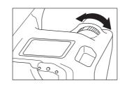
\* The shutter speed of some Canon cameras changes automatically if the shooting mode dial is set to Av and the brightness is set by turning the aperture ring. Therefore the shutter speed is not required to be set additionally as with the M
