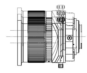
The shifting knob is black and the locking knob is grey. Use the black knob to adjust the shifting and rotate the grey knob in L direction to hold it in place.
