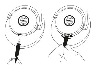
**To detach cable:** Turn the plug COUNTERCLOCKWISE a quarter turn and remove it from the jack.
