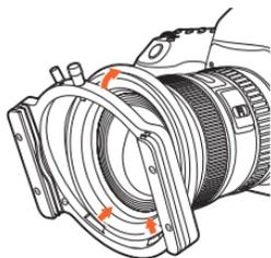
3. Align the filter holder with the adapter ring so that the locking pin is on top, and the film clips face away from the camera.
