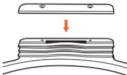
4. Replace the top clips by placing them on top of the newly added clips. As in the previous step, make sure the curve is oriented similarly with the other clips.
