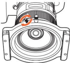
7. For additional security, tighten the locking screw by turning it clockwise.
