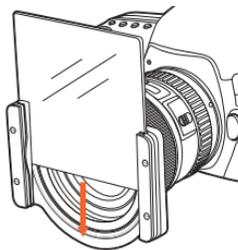
8. Install a filter into the holder by sliding it into position between the film clips. Due to the snug fit, the filter may have to be slightly jiggled to glide into the clips.
