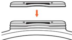
2. Remove the top clips and insert the extra film clips by placing them under the top clips.
