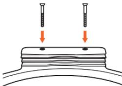
5. Replace and securely screw in the clip screws. If it is taking too much effort to insert a filter, check the orientation of the clips to make sure they are all curving in the same direction.
