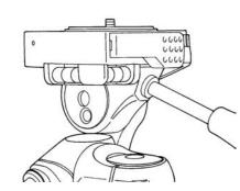
Two bubble levels are built-in for vertical and horizontal positioning.
