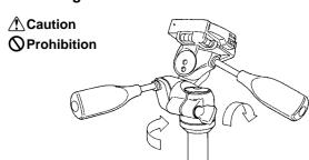
Set the new head, or accessory on the tripod's threaded post, and turn clockwise until it comes to a stop. Tighten the Panning Lock Knob and turn clockwise slightly more.
