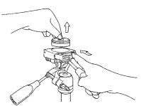
Remove Quick Shoe by opening the Locking Lever and then pressing the Release Button.
