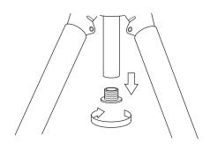
Remove the Center Column Base Stopper truning to the way of arrow.
