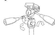
Please exchange by the following method to attach other heads or accessories to this leg. Fix the Center Column of the legs firmly by both the Center Column Locking Collar and the Center Column Stopper. Next, tighten the Panning Lock Knob of the head firmly. The Pan & Tilt Handle and the Vertical Tilt Handle are grasped and then, turn the head counterclockwise forcibly. The head loosens now.
