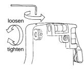
After long use, you may need to re-tighten the Lever Lock mechanism through the window located underneath the Pan Head. First, you will need to loosen the locking pin
