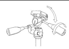
Loosen the Vertical Tilt Handle, and the level can be adjusted.
