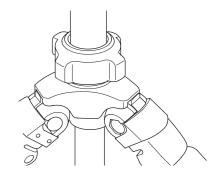
After choosing the desired leg angle, securely push in the Adjustment Lock.
