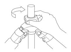
Insert the Center Column from the lower side of Main Body, and tighten the Locking Collar and the Center Column Stopper.
