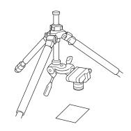
By inverting the Center Column, it is possible to do copy, and close up work.
