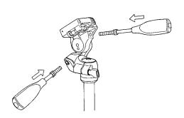
Attach the two Pan Handles to the Pan Head, by inserting the shorter handle to the left, and the longer horizontal tilt handle to the right. Do not reverse.
