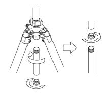
Remove the Center Column Base Stopper and then, remove the Lower part of Center Column. Put the Center Column Base Stopper on the Upper part of Center Column.
