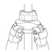
To change the angle of each leg, close the Leg slightly, and then pull the Leg Angle Adjustment Lock out. There is a choice of two other angle positions
