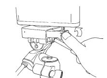
Fix the Quick Shoe at a desired position by closing the Locking Lever.
