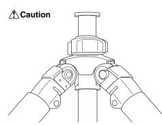
Make sure to re-attach the Center Column Base Stopper, in order to prevent the Center Column from falling out.
