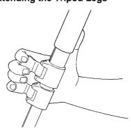
Flip up the Leg Lock Lever to extend or shorten any of the individual leg sections to the desired length, and press the Leg Lock Lever flush against the Leg to lock.
