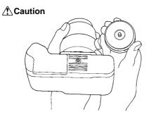
Screw Quick Shoe on to camera, and insert back into the Camera Platform. Please DO Not over tight your Quick Shoe.
