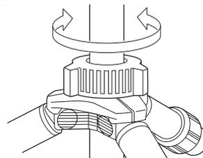
Loosen the Center Column Locking Collar by turning it counterclockwise. Raise the Center Column to the desired height and lock in place by turning the collar clockwise.
