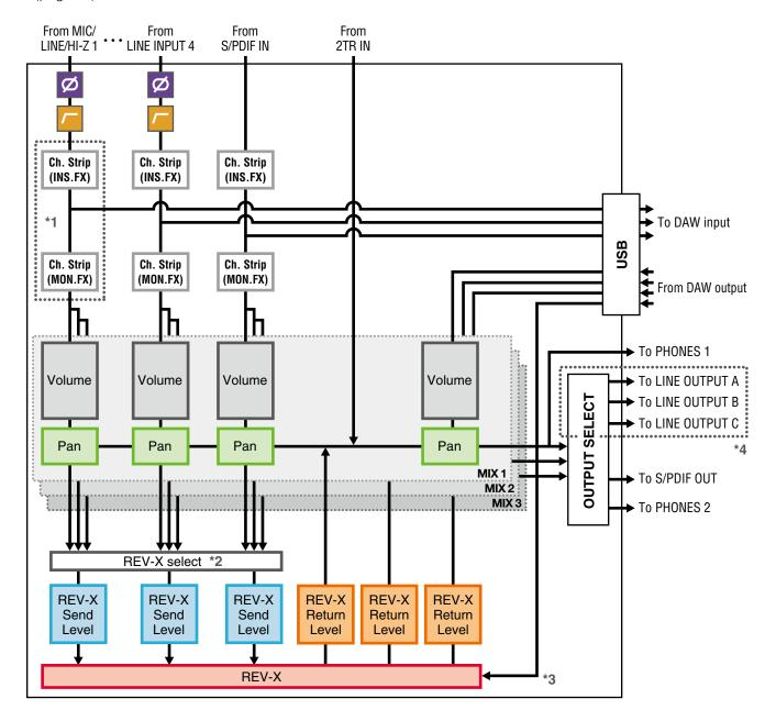
\*1The following chart indicates the Ch.Strip (Channel Strip) insertion location.
