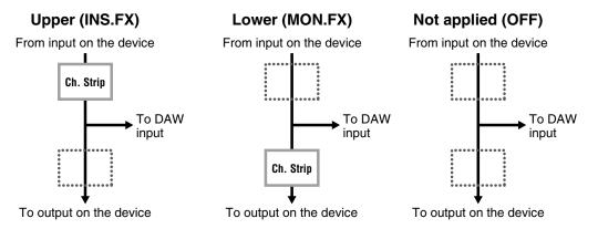
You can apply four Channel Strips to mono channels, or two Channel Strips to a stereo channel.
