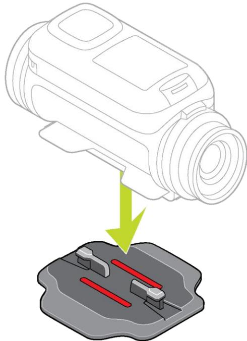
3. Make sure the mount is aligned in the correct direction, then, in dry, room-temperature conditions, attach the mount. Push the mount firmly down onto the surface. The mount won't attach securely if you install it in damp and cold conditions.
