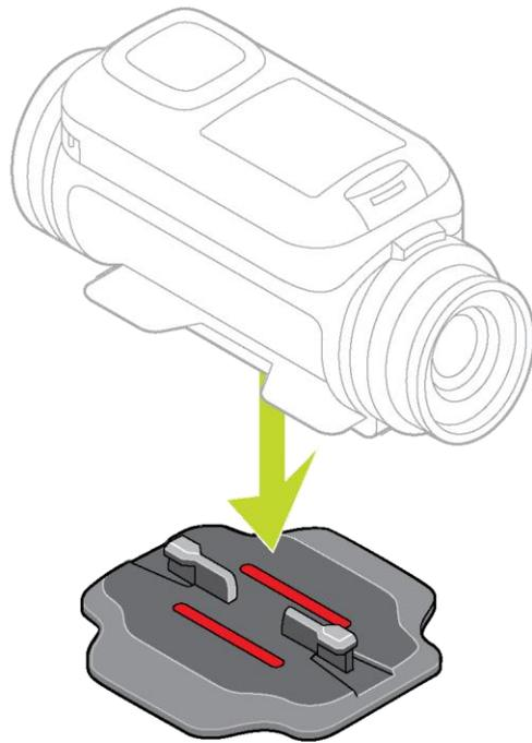
3. Make sure the mount is aligned in the correct direction, then, in dry, room-temperature conditions, attach the mount. Push the mount firmly down onto the surface. The mount won't attach securely if you install it in damp and cold conditions.
