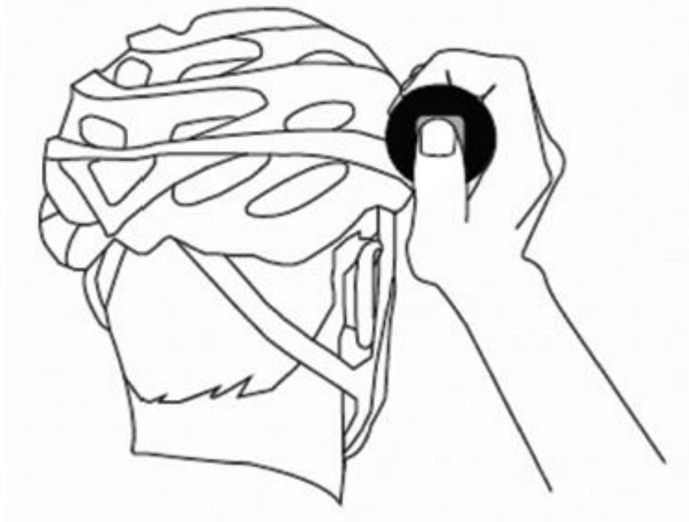
1. Before you install a mount, find the best position for your TomTom Bandit. Only attach the mount to a smooth, hard surface. The mount won't securely attach to porous, textured or soft surfaces. To install the TomTom Bandit at different angles and on the left or right side of a helmet, you can turn the TomTom Bandit's base more than 180 degrees around the TomTom Bandit body.
