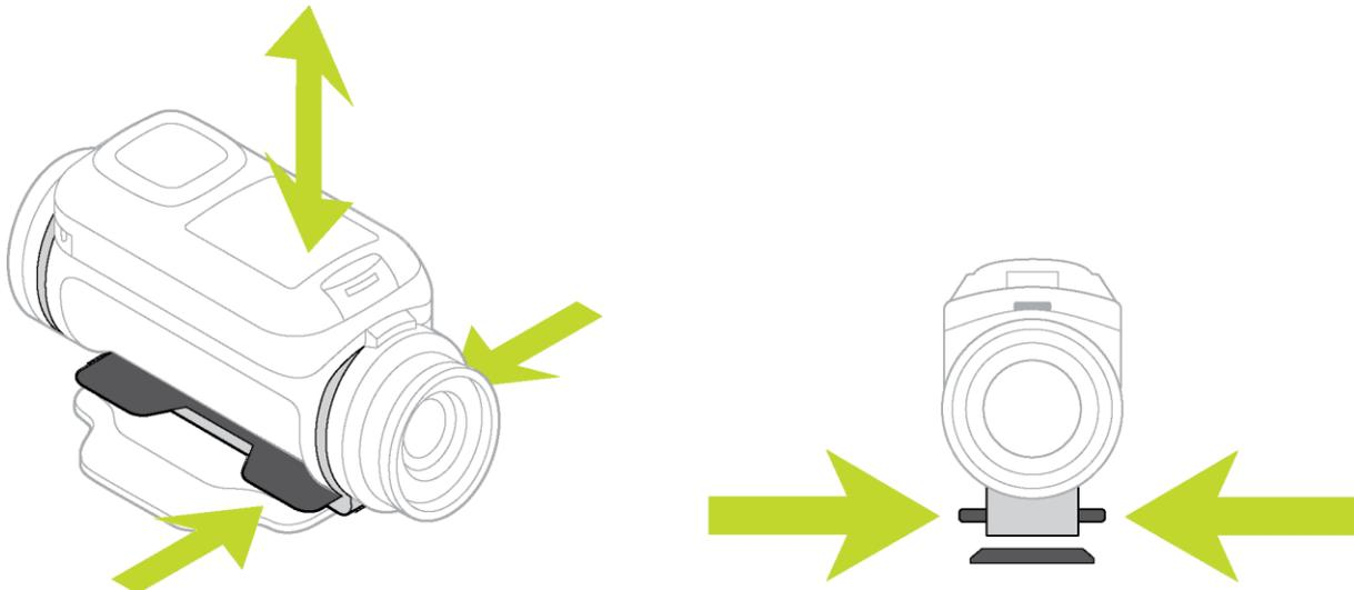
7. Adjust the position of the TomTom Bandit, then push the pitch mount lever to the closed position to lock the pitch mount.
