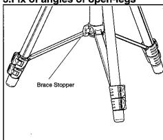
When opening legs, loosen Brace Stopper and open legs to the maximum. Secondly, tighten Brace Stopper in order to fix the angle of openlegs. If the place does not allow to open legs, do not try to use the tripod. The tripod may fall.
