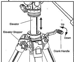
Rotating the Crank Handle for Up and Down the Elevator after unlocking the Elevator Stopper. Locking the Elevator Stopper tighten when reaching the desired height.
