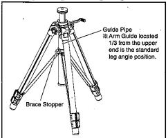
Loosen the Brace Stopper to open the Leg angle. The standard Leg angle located at 1/3 from the upper end of the Guide Pipe.
