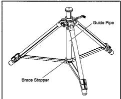
Lower the Brace Stopper at the end of the Guide Pipe, Semi Low position is available for the tripod.
