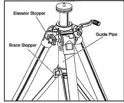
Brace Stopper is to adjust the friction of the Elevator to loosen or tighten.
