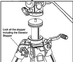
In order to remove the Head to change, lock all the stoppers on the Head and The Tripod. Then turn the whole unit of the Head toward anti-clockwise direction as the arrow showing. The tripod screw is 1/4 inch. So please choose the Head having the 1/4 inch screw at the bottom of the head.
