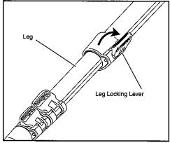
Flip up the Leg Locking Lever by the thumb of the right hand. Then extending or folding the leg to the desired length, then Locking the Lever tighten firmly. Use upper Leg section when using in the middle way of the whole length. Upper Legs have
