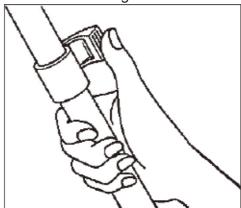
Using thumb to open the Leg Locking Lever to extend legs to the desired height. Then locking each leg section firmly. For the folding legs, opening the Leg Locking Lever and collapse from the lower leg section to the upper leg section.
