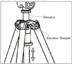
Unlocking Elevator Stopper, extend the Elevator to the desired height. Then lock the Elevator Stopper. Hold the Elevator tightly while extending or closing down otherwise it may suddenly come down to damage your camera or harm your fingers. Be careful.
